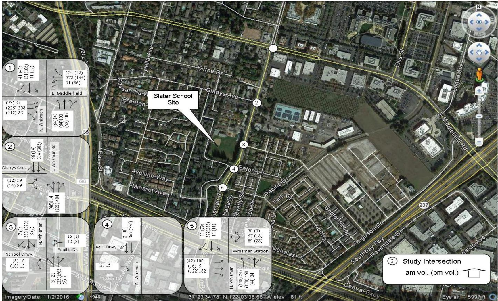
Figure 4 Current (2017) Conditions School Peak-Hour Traffic Volumes Slater Elementary School Traffic Study-Mountain View
