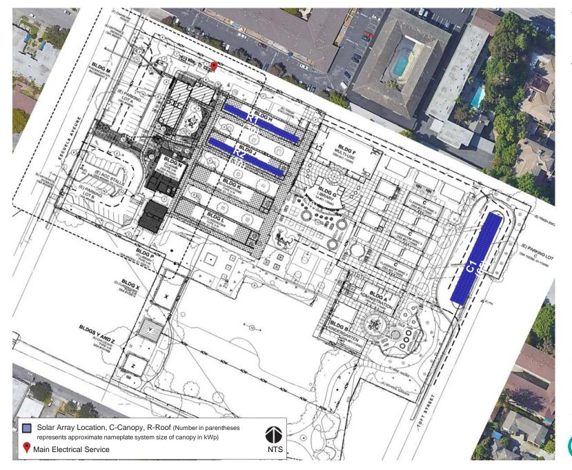
Target PV - 125 kWp PV Shown - 125 kWp (100%)
